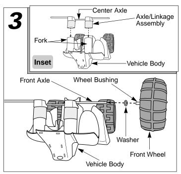
**Please Note:** If the axle/linkage assembly has detached from the vehicle body during shipment, please fit it back onto the fork on the front of the vehicle body. Make sure the center axle is toward the rear of the vehicle.
